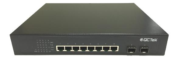
PG-08 series, a 10-port Gigabit PoE+ Switch, is a standard Gigabit Ethernet switch that meets all IEEE 802.3/u/x/z/ab/af/at standards. The switch includes 8-Port 10/100/1000Mbps RJ-45 with PoE+ function and 2-Port Gigabit SFP for Fiber. It is an ideal solution for applications of wireless AP, IP phones and IP cameras.
